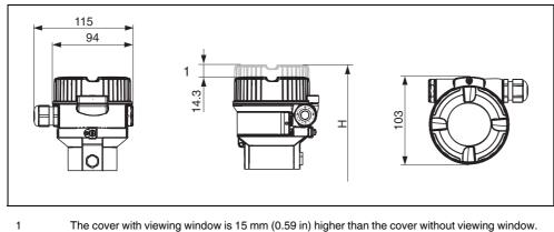
The cover with viewing window is 15 mm (0.59 in) higher than the cover without viewing window.
