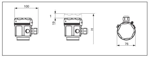
1 The cover with viewing window is 19 mm (0.75 in) higher than the cover without viewing window.
