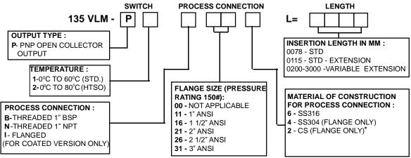
\*Note: Slip on Flange with suitable threading in required material e.g. CS/SS316/SS304, will be provided for all Flanged versions except coated.
